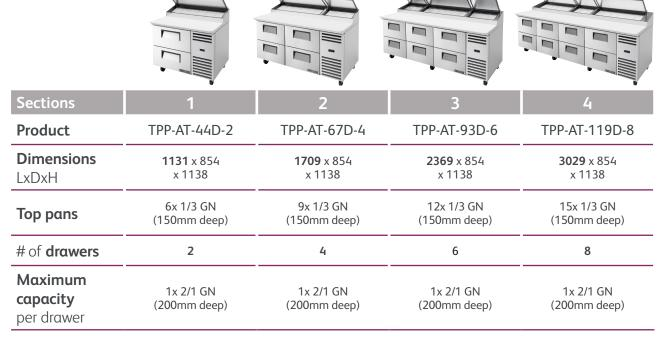
Depths do not include 73 mm cutting board overhang or 26 mm for rear bumpers.
