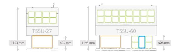
As standard, TSSU products are not supplied with any drawer divider bars. Drawers accommodate 1x1/1 or 3x1/3 pans without the need for additional bars.
