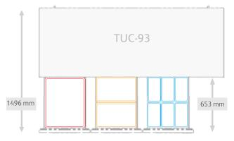
Deep TUC 67 & 93 products are supplied with 1 horizontal divider bar per drawer, facilitating 2x1/1 pans, 6x1/3 pans, or a combination of.
