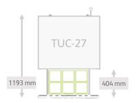
TUC 27 & 60 feature internally integrated refrigeration systems, accepting 1x1/1 pan per drawer, ideal for operations where space is limited.
