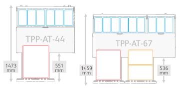
As standard, TPP products are supplied with 1 horizontal divider bar per drawer, facilitating 2x1/1 pans, 6x1/3 pans, or a combination of.
