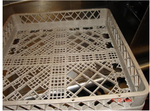
Damaged and broken rack that will jam or skip conveyor
