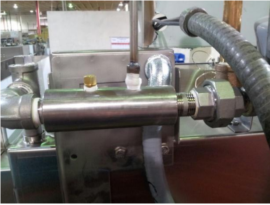
Mixing chamber with two 1/8" pipe threaded ports Hi-temp mixing chamber is SS, Chemical is a polymer
