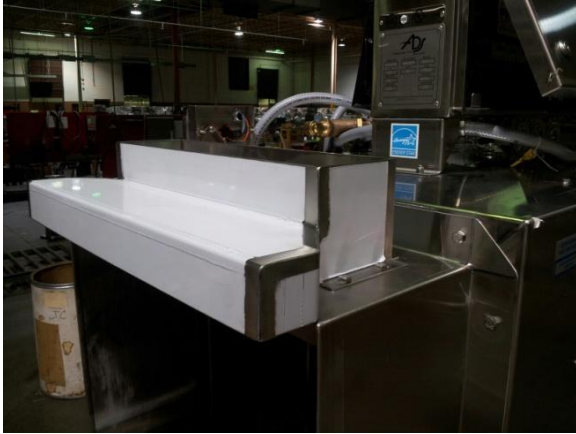
Vent attachments to end shield, 4" x 16" opening
