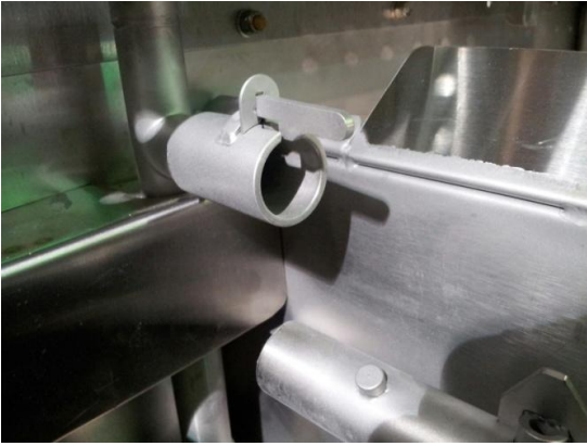
Showing pumped rinse manifold locking tab
