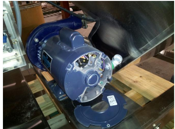
66 power scrapper motor, 1.5 HP, 208v, single-phase
