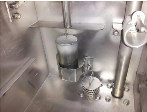
Rinse tank float, pump filter, pumped rinse manifold
