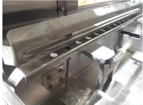
Wash tank sequence bar, pendulum with magnet
