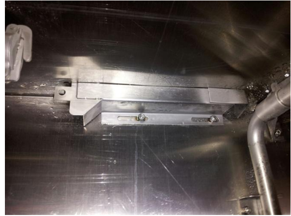
Diverter plate separates fill stream for wash and rinse tank
