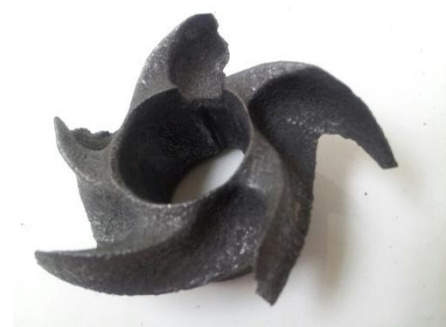
Impeller damaged from high acid solution
