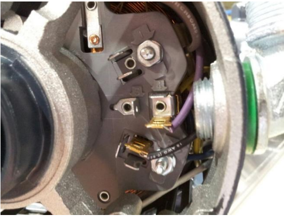
Showing connection points in 1.5 HP, 120v motor black & white wires attach to spades left of two nuts
