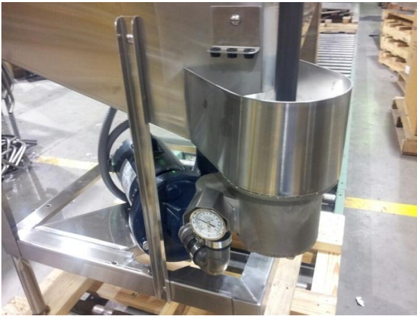
Showing AF-ES sump, drain ball, thermometer
