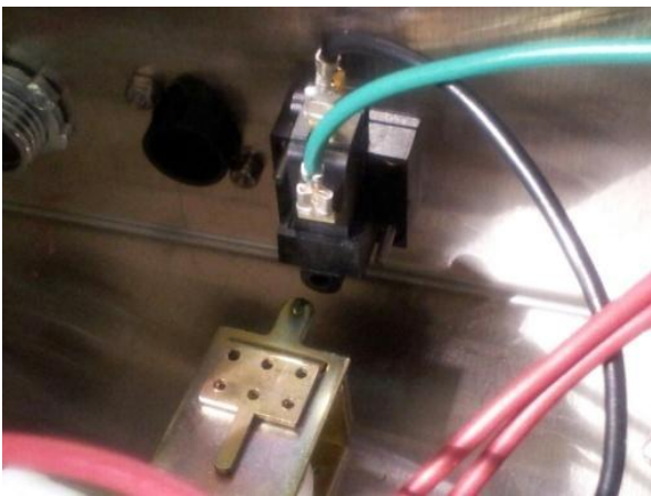
OPTIONAL Chemical Alarm switch, buzzer
