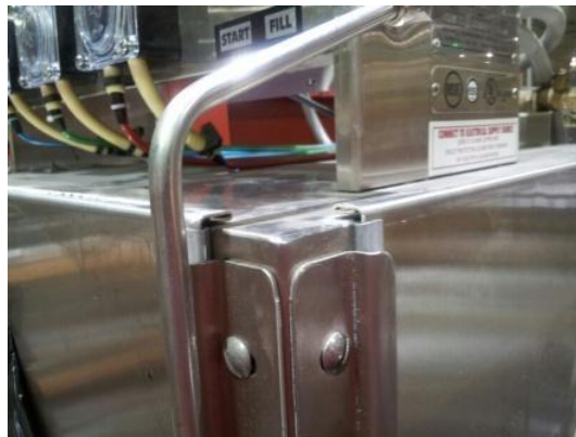
Showing correct arm alignment
