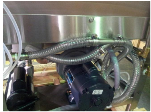
Drain "y" from overflow & drain pump, 48" drain tube
