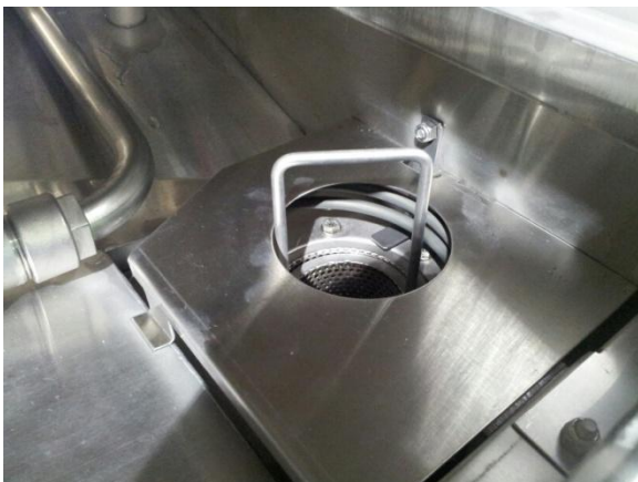
Sustainer heater cover and pump filter system
