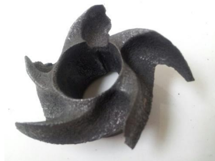
Impeller damaged from high acid solution
