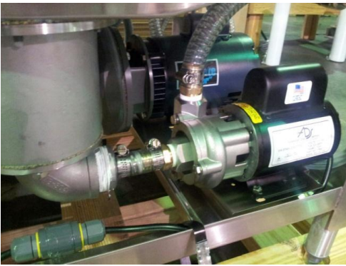
Showing stainless drain pump w/3/4" discharge tube
