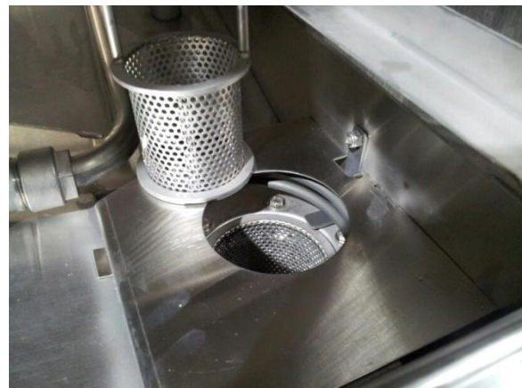
Secondary basket for dumping, primary filter shown in place
