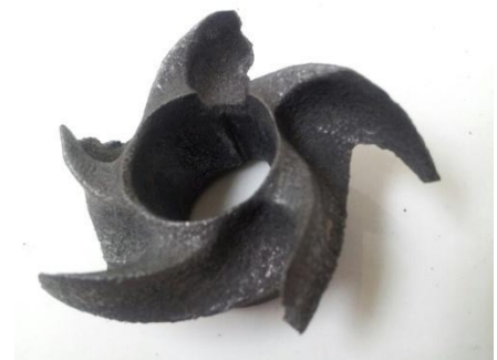
Impeller damaged from high acid solution
