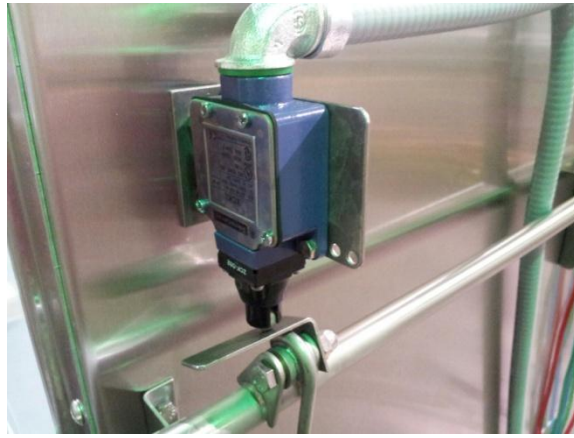
5AGES Door cut-off switch and lever arm
