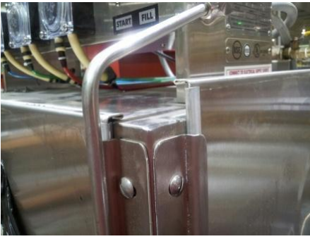
Showing ❌ misaligned arms on corner
