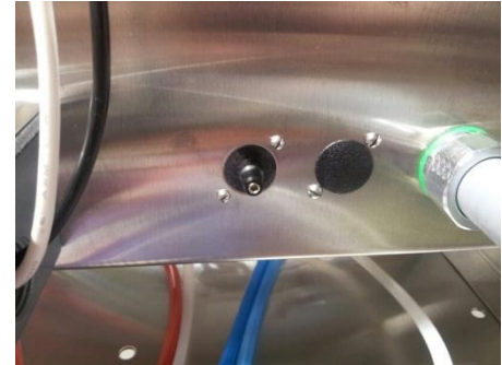
Chemical alarm barb adjusting screw *
