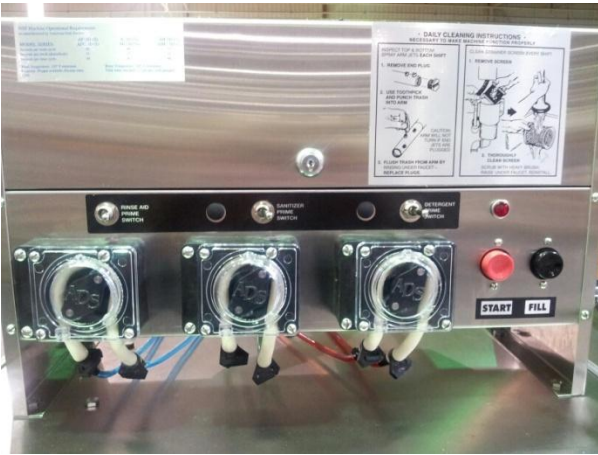
Showing the control box with chemical pumps prime switches, red start and black fill switch
