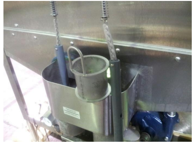
5AGES sump, drain balls and stainless filters
